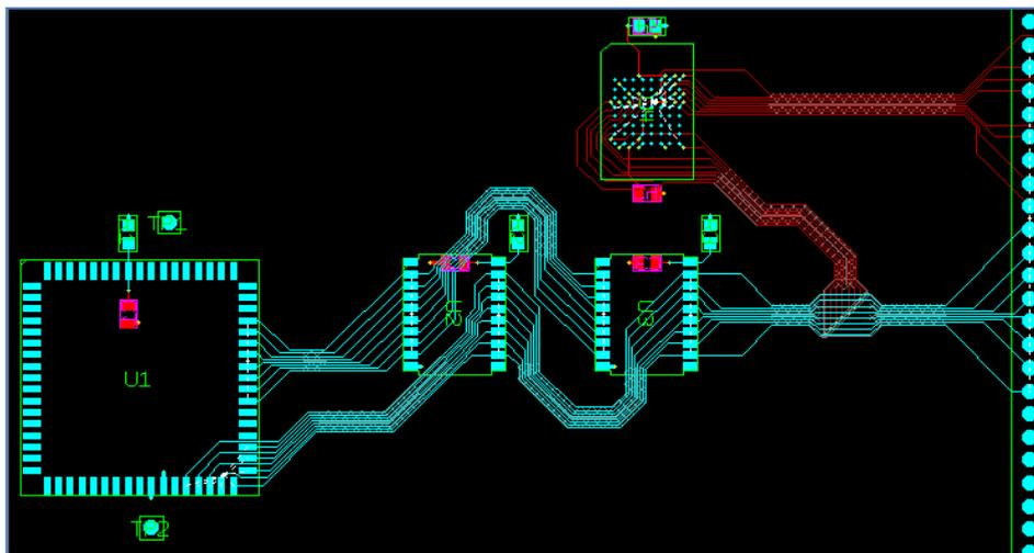
Trunk Routing, Manual and Activ-45 routers to interactively route the connections up to the end and finish the board.
