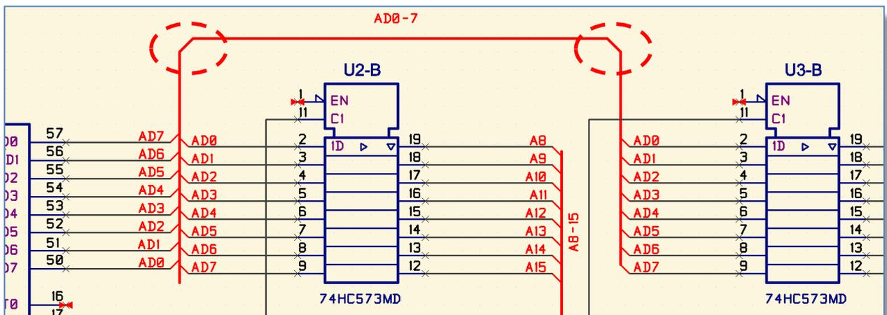
**Tip:** Add Mitres to the bus corners using the **Mitre Corner** function located on the [Net/Shape] tab.
