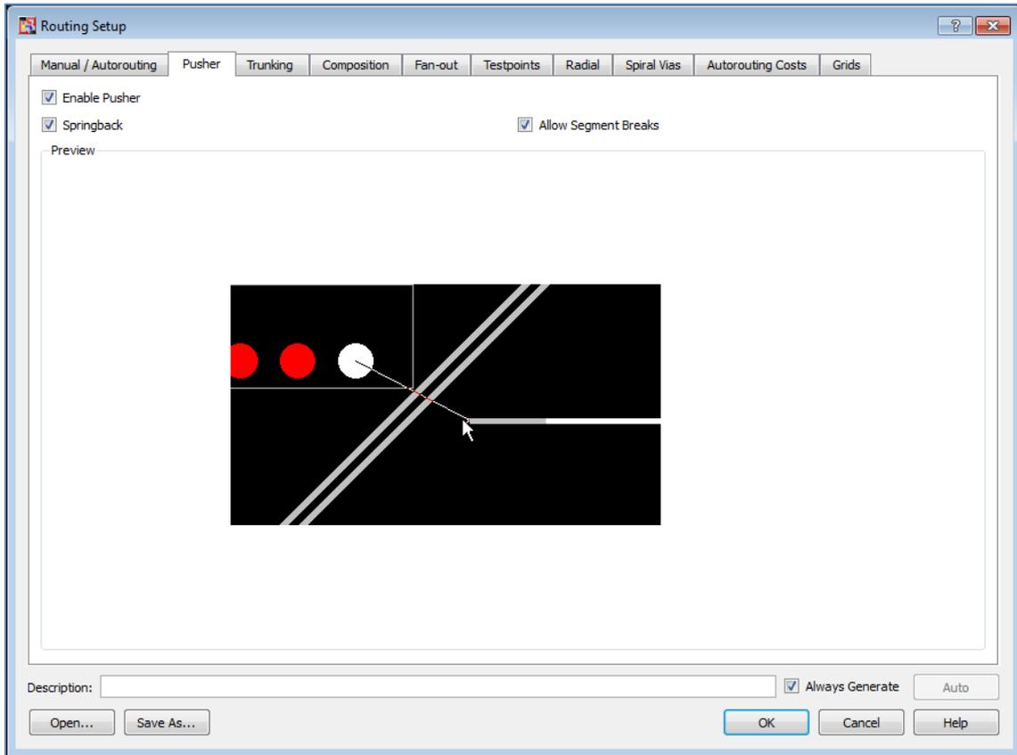
P.R.Editor can also be used for placing components without going back to the Design Editor. Before starting any placement check the **Interactive Move** and **Push Aside** options.
