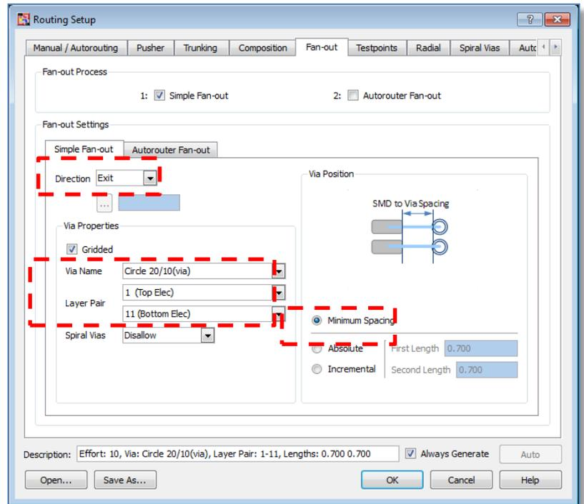
14. Select **Routing**→**Fan-out**→**Perform Fan-out** or click the icon
