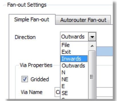
10. When you are happy with the Fan-out you can save it for reuse, by selecting **Routing→Fan-out→Save**
