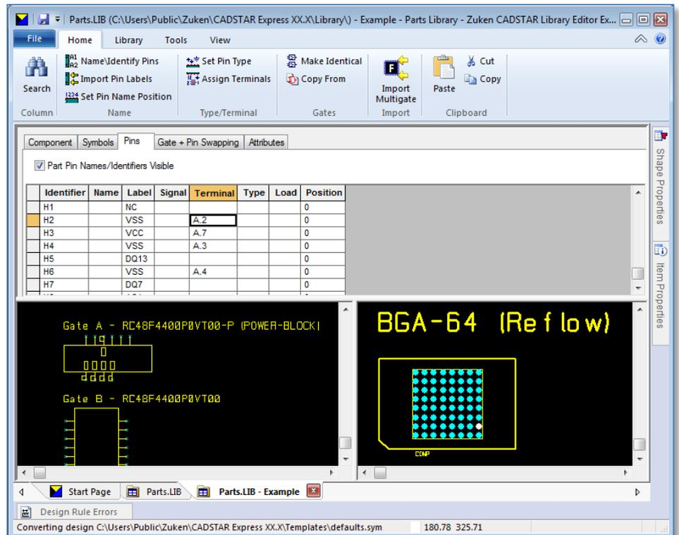
Continue assigning the terminals for Gate B (*RC48F4400P0VT00*). Just click in the terminal field of pin A1 (Label A1) and you will notice that automatically B.1 = {Gate B.Symbol Terminal 1} will be assigned.
