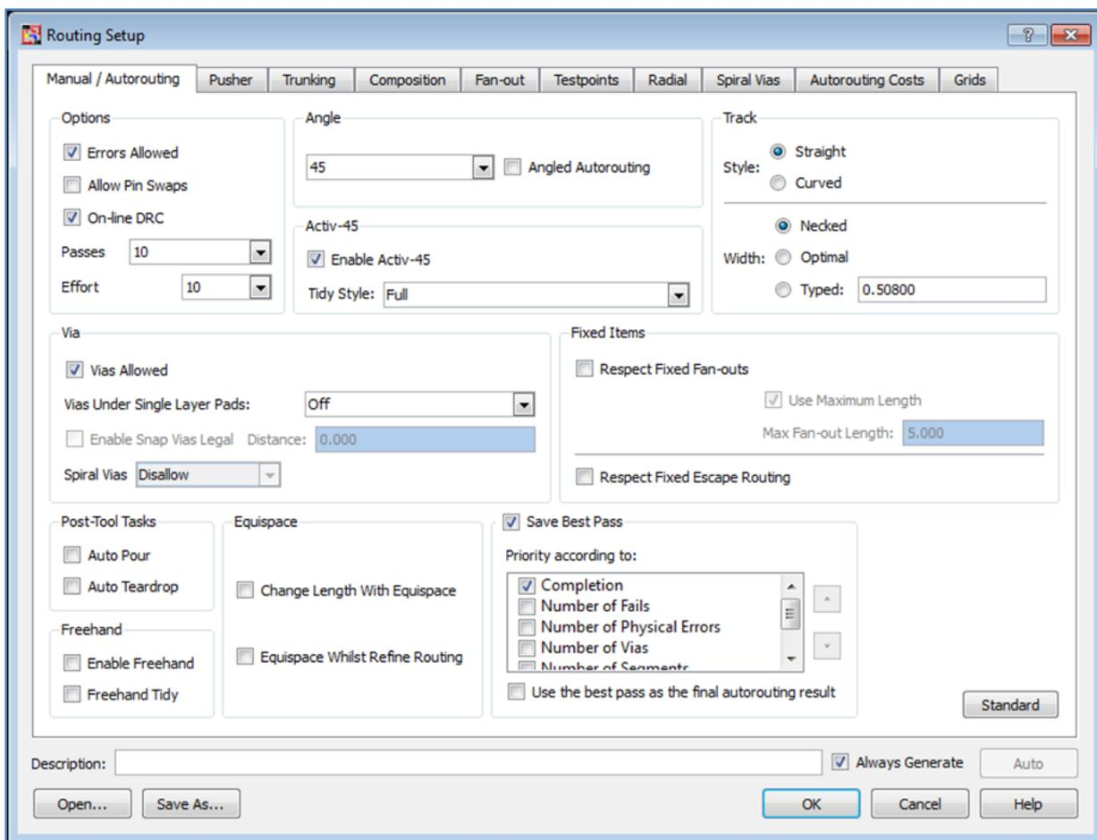
**Note:** Although errors are allowed, you should first allow the router to make some errors. In combination with Effort 10 the router will continue routing till no errors are left.
