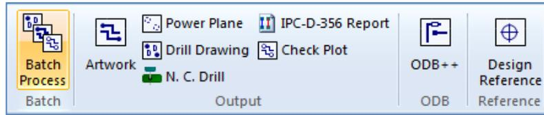
If you like, you can create the manufacturing data for this design by selecting [**Manufacture**] tab → **Batch Process**. In the Batch Process window select [**Open**] → **Manufacturing Output 6 Layer.ppf**, which you can find in the Self teach directory and click [**START**].
