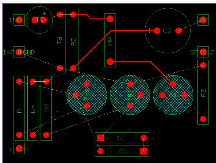
5. Now route all the connections on Bottom Elec layer and insert jumpers if necessarily.
