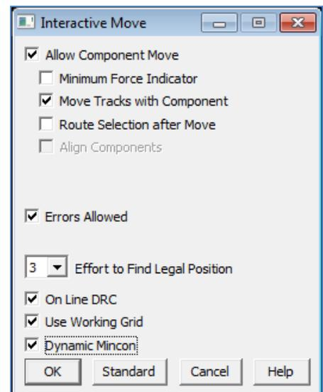
3. Select **Configure**→**Placement**→**Push Aside** in the menu bar. Ensure the settings are equal to the example.
