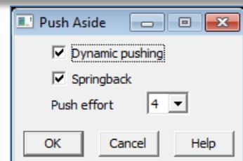
4. Select a component and click the **Move** tool bar icon . Notice that other components are being *pushed aside* and when there is enough space the selected component jumps over other components. Components can also be swapped to the other side of the board or rotated . This can also be performed using the **<R.M.B.>** assist menu.
