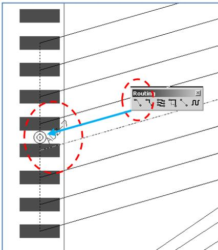
← Busses of data and address lines can be pre-designated in a schematic design (as done in DesignC) and transferred to PCB and Place & Route Editor XR. A named bus (trunk) can be selected by its' bus marker.
