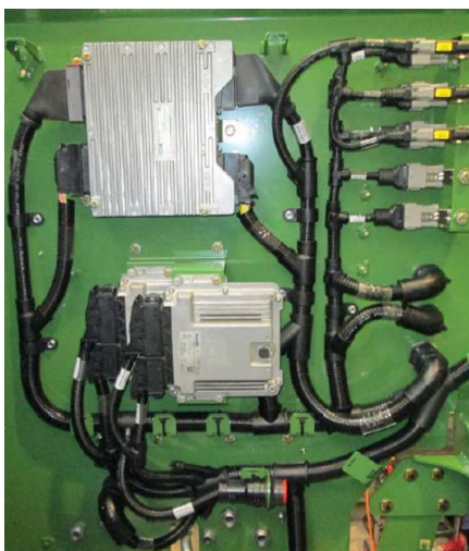
Comparison of the 3D harness design in MCAD with a photograph of the physical product.
