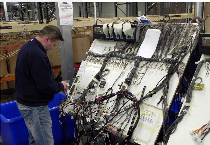
*Figure 2: Every cable harness is fully tested. Before switching to E<sup>3</sup>.series, which is tightly integrated with BCA Leisure's ERP, repeat faults were being found as a result of applied fixes not being back annotated to the schematic. Now, strict version control is in place - and unless the schematic is correct the harness cannot be made.*
