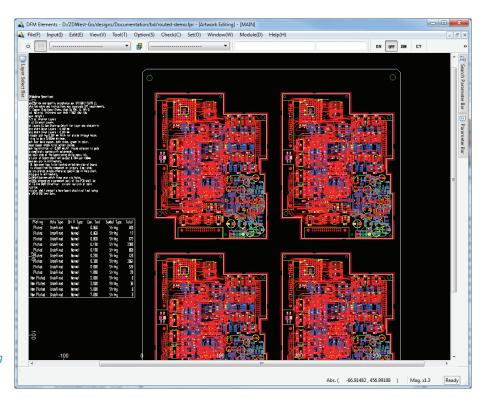
DFM Center is a comprehensive manufacturing preparation and output solution supporting panelization and common output formats.
